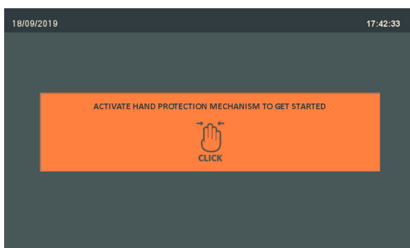
Fig. 31 TFI Hand Protection Guard Check Screen
