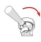
Insert the portafilter and rotate it counterclockwise until the handle is approximately perpendicular to the face of the coffee machine.
