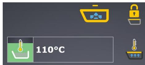
During this process, the information panel shows indication of the steam flow
