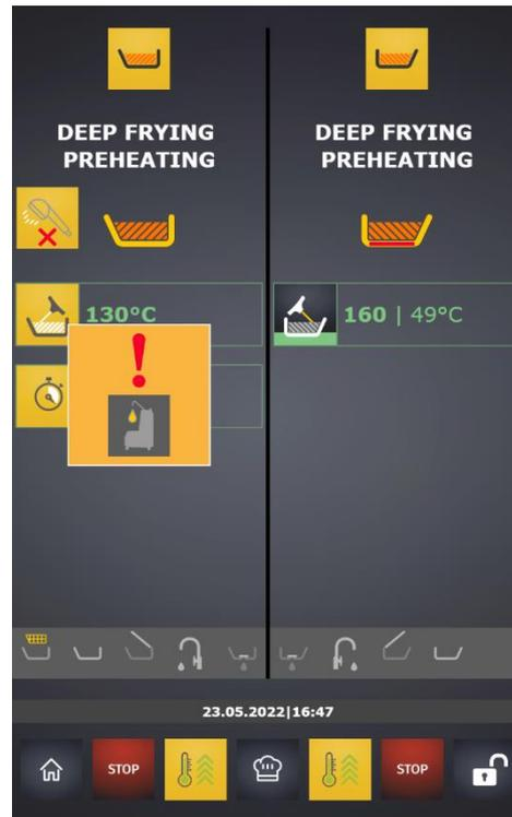
Temperature interval MAX – MIN for deep frying mode is 180 - 130 °C
