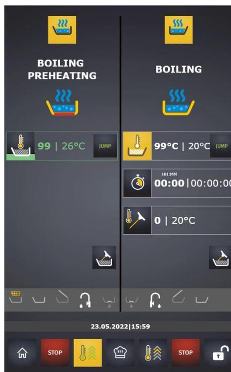
Temperature interval MAX – MIN for boiling mode is 99 - 30 °C.
