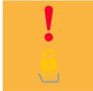
alert – the cover is not locked in the end position when the pressure cooking is switched on or the cover is not unlocked in the end position when a mode other than pressure cooking is selected
