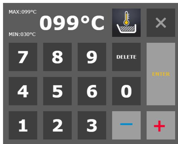
The displayed MAX and MIN values determine the interval in which the value can be entered. If you choose a value outside this interval, the maximum or minimum possible value is chosen. The set value appears in the upper field. The type of temperature control is displayed at the top right.
