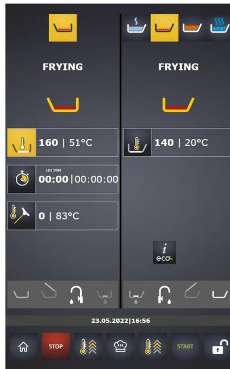
Temperature interval MAX – MIN for the frying mode is 250 - 60 °C.
