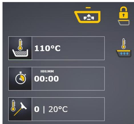
After entering the time or core temperature, heating takes place to the required pressure-cooking temperature.
