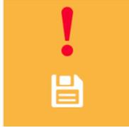
alert – the SD card is fuller than the set occupancy (service parameter) or the device memory is being read/written
