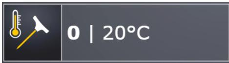
heating is not switched on and the required core temperature can be set
