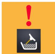
warning - the probe is not inserted into the pan, i.e., the temperature difference of plate 1 or plate 2 respectively is greater than 80 °C compared to the minimum temperature on the probe
