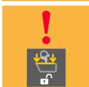
alert – signalling of the need to push on the cover of the pressure pan to release the cover lock
