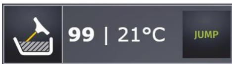
heating is not switched on in the pan temperature control mode according to the probe
