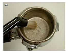
Remove the sprayhead weekly and thoroughly clean the filter and its holder.
