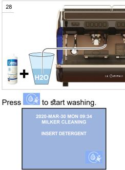
At the end of the first washing phase, connect the Milker circuit to a container with clean water for rinsing.
