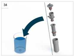
Brush the Milker dispensing nozzle with the brush to remove the residues.
