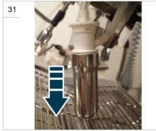
Disconnect the connection hoses of the milk circuit.
