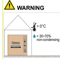
In case of prolonged storage at temperatures below 2°C, the water circuit in the machine must be drained by the Customer. Do not switch the machine on before having reconditioned it for at least 1 hour at a suitable room temperature. If it is installed in areas with room temperature above 30 °C, malfunctioning may occur.
